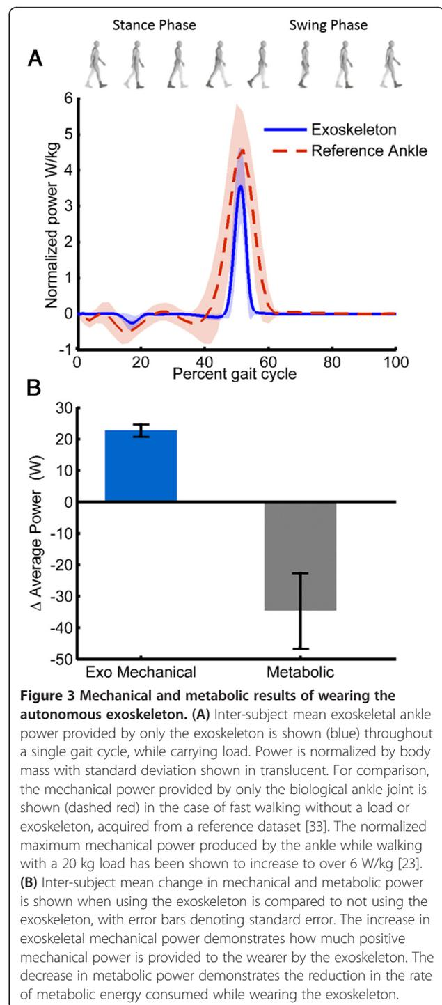
The lightweight architecture of the exoskeleton allowed it to add positive mechanical power to the user without restricting the natural motions of the ankle joint. In order to apply a large torque about the ankle joint, it must be reacted by both a structure connected to the foot and a structure connected to the shank. Applying large forces to the body must be done carefully, in order to prevent discomfort or pain. One solution is
