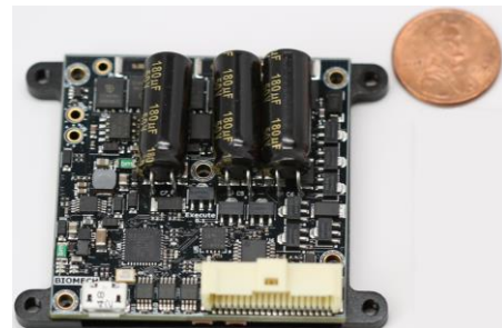
Figure 1 FlexSEA-Execute 0.1 mounted on its optional heatsink
