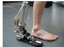
Fig. 1 A prototype of the robotic ankle-foot emulator.
