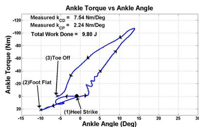
Fig. 2 Measured ankle torque-angle plot of the emulator of one gait cycle. The plot began at heel-strike and ended at toe-off of the gait cycle. The area enclosed by the curve represents the work done at the joint. The amputee’s walking speed was dramatically increased in the experiment because the emulator added an additional amount of mechanical energy into the body in each gait cycle.
