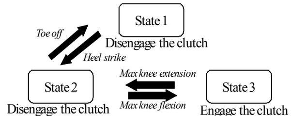
Fig. 6 The AG state machine controller. The clutch is engaged only after maximum knee flexion in the stance phase. The clutch is disengaged automatically when the spring releases all stored energy. consumption and carbon dioxide production and calculated metabolic rate [9].
