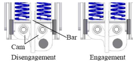
Fig. 5 Clutch mechanism. When cams are disengaged, the bar can move up and down without any resistance. When cams are engaged, the bar moves up under spring force, (but down without the force).
